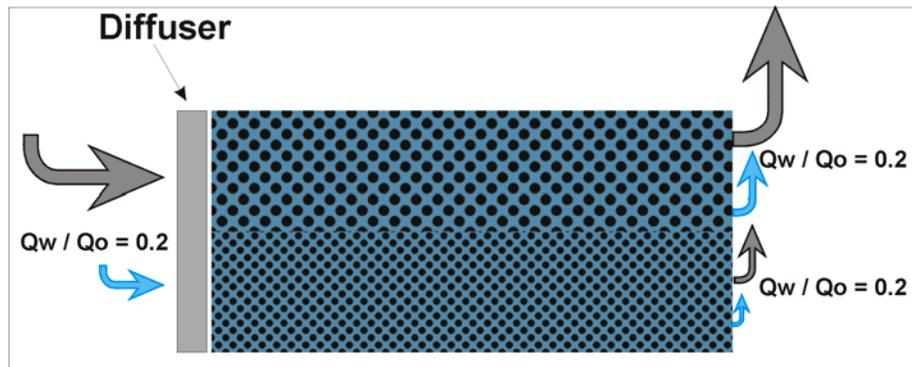
Fig V-11: Both layers at steady state condition and producing proportionally to their permeabilities ratio.
