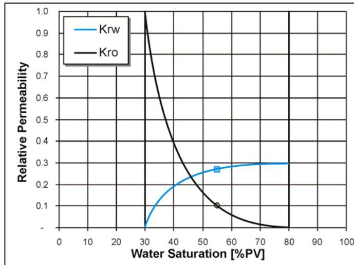
Fig. V-7: “Relative permeability curves” in unsteady-state displacement for the entire block in Fig. V-1.
