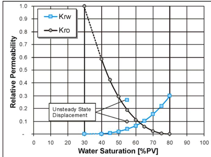
Fig. V-6: Relative permeability values calculated for unsteady-state displacement. Calculated points fall far apart from original relative permeability curves.
