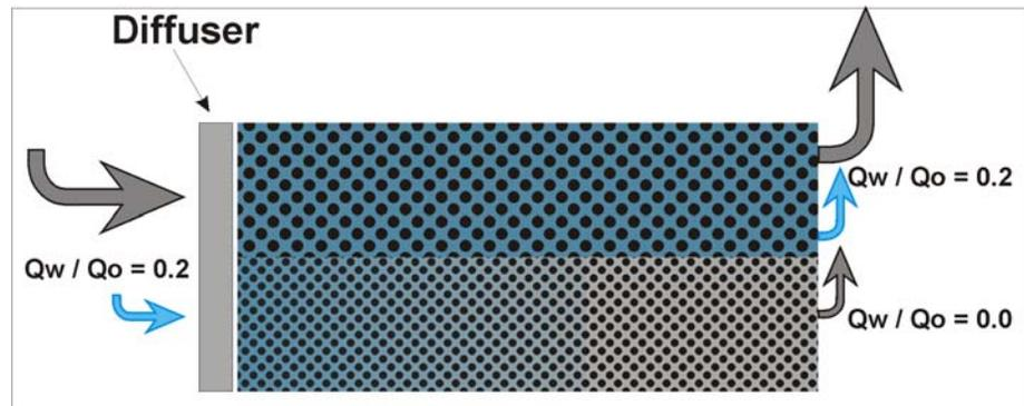
Fig V-10: The most permeable layer reaches steady state while the less permeable layer is still in transient state.
