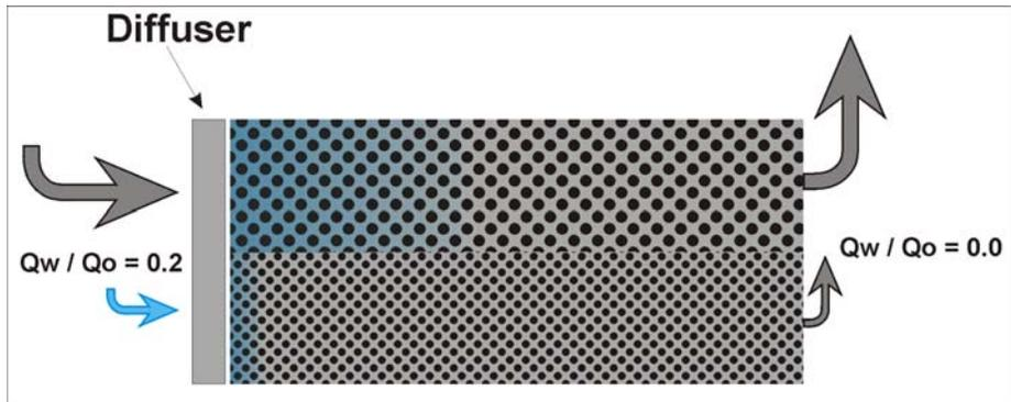
Fig. V-9: Both layers receive water and oil but at a rate proportionally to its own permeability.
