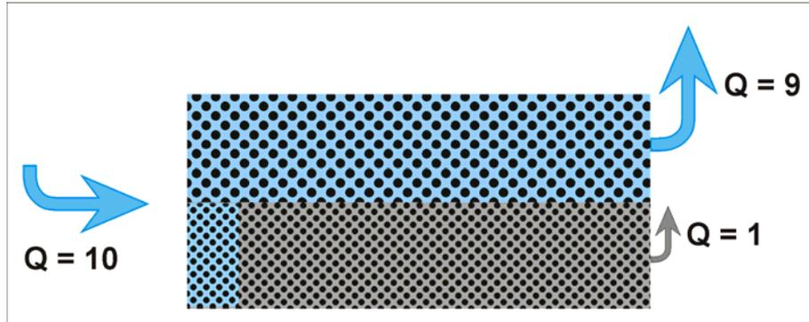
Fig. V-5 Water has reached the output face (Breakthrough). The less permeable layer still produces oil.
