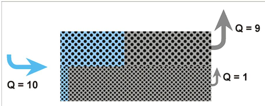
Fig. V-4 – Advanced stage of water injection from the left. Water (blue) displaces oil (gray) at different rates in each layer.
