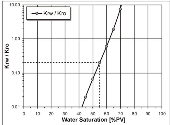
Fig. V-8: Relative permeabilities ratio corresponding to “experimental” curves in Fig V-2.  $K_{rw} / K_{ro} = 0.2$  ratio is obtained for  $S_w = 55\%$  PV
