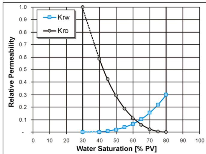
Fig. V-2: The same water-oil relative permeability curves for both layers in Fig. V-1.
