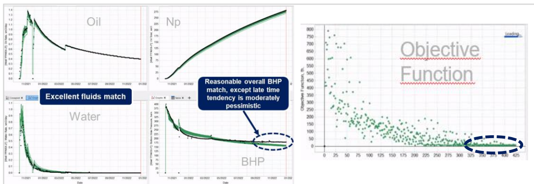
Fig.-12 – 1 st Loop matching results (Left: 30 best OF runs) – (Right: Objective Function convergence chart vs number of runs)
