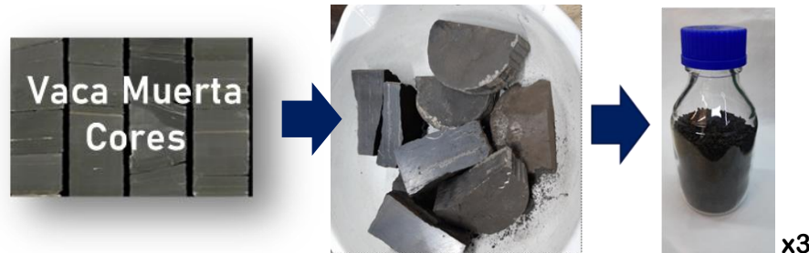
Fig.-3 – Lab procedure to generate the crushed rock sample
