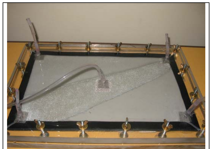
Fig. 2: Injected gas saturation is appreciable through Zone 1. Water goes out from Zone 2 production end.
